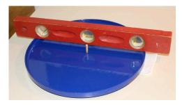
Use the spirit level to make sure the mold is as close to level as you can get it. If necessary, use folded paper towels as shim. Check the level from front to back and from side to side. Any departure from true level will result in a disk that is thicker on one edge than on the other.
