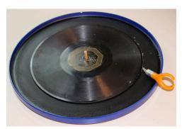
Place the real 78 over the wax disk, with the short dowel sticking up through the hole in the 78. Use the X-Acto knife to cut straight down all around the rim of the 78. (Unavoidably, this is where the mold gets scratched.)
