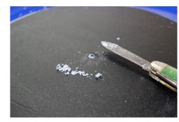
Use a cloth rag to polish the top (less shiny) surface of the wax disk a bit. At least do it near the hole, because otherwise the tape for the label won't stick.
