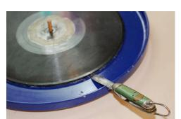
Once all the scrap has been removed, it's time to separate the wax disk from the mold. This is the point at which you need to
