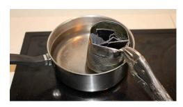
Put a couple of inches of water into the water pot and place it on a stovetop burner. Put wax granules or pieces into the can, and put the can into the pot. (In the illustration, instead of wax granules, the can contains wax pieces left over from a previous session.) Turn the heat to high initially, and then turn it to medium-low when the water is almost hot enough to boil. Assuming a 12-inch mold, you should aim for about one cup (fluid volume
