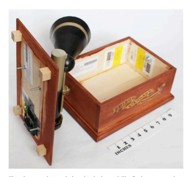
This phonograph is made from birch plywood. The flat base was ready-made, probably intended for making a plaque. It was about the right size, so I let it determine the other dimensions, except that the height of the four sides was determined by the width of available hobbyist plywood. The small black plastic base was a sort of tray thing I had lying around.
